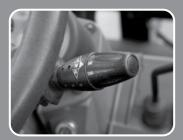
**Multi-function switch lever** Multi-functional switch lever gives easy access to lights and turn sign lamps.
