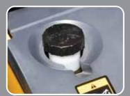
Brake fluid reservoir Highly visible, easily accessible reservoir makes quicker daily inspections.
