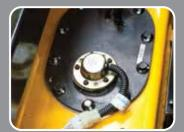
**Fuel tank safety valve** Integrated safety check valve shuts off fuel supply in the unlikely condition of a truck overturn.
