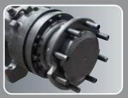
Wet disc brake system The wet disc brake system is virtually maintenance free and is enclosed to protect from dust and water.
