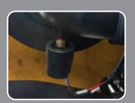
Electrically monitored air filter Air cleaner sensor alerts the operator
