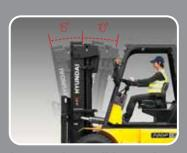
**Increased mast tilting angle** The mast tilting angle of 15 degrees forward and 10 degrees backward, the operator can safely and rapidly perform loading and unloading jobs.
