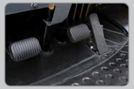
**Ergonomically positioned pedals** Based on human engineering, the accelerator, brake and inching pedals are optimally positioned for convenience while operating the equipment.
