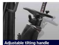
The handle angle can be adjusted with the lever on the right side of the steering wheel to suit the operator's physique and driving habit.
