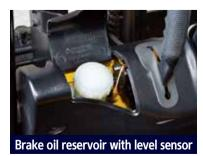
The enhanced brake oil reservoir, located in the upper left dash is equipped with an electronic level sensor that shows the level in the LCD color monitor.
