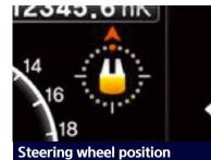
A steering sensor is applied to the king pin of the rear axle, communicates to the LCD color monitor to show the direction of the vehicle as it relates to the angle of the steer wheel.
