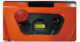
Battery deep discharge protection device, voltage discharge indicator with low voltage automatic cutting and lifting function, for higher battery lifetime.
